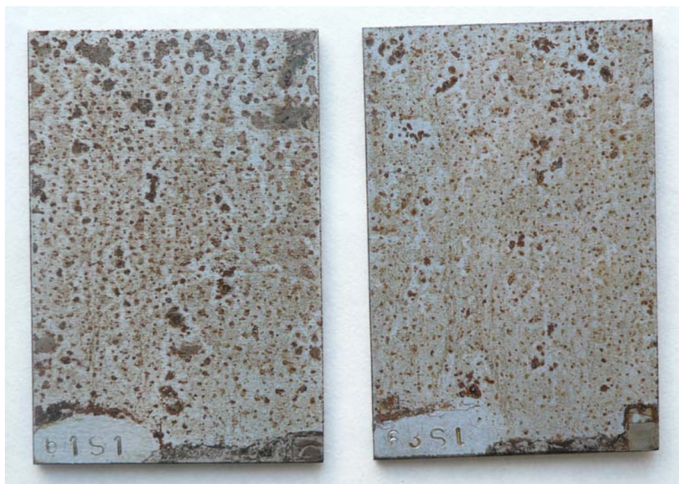
Fig. 1 Aspect of the steel specimens of set 2, after pre-corrosion, partial cleaning and coating
